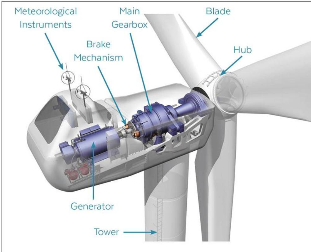
Figure 4-3 Turbine nacelle and-5 hub components
