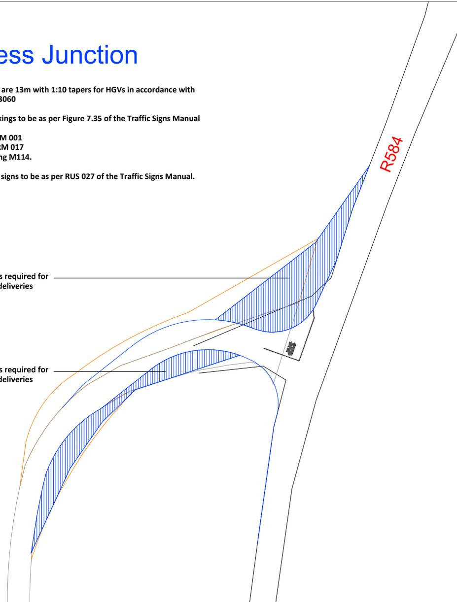
Figure 14-15 Access Junction on R584, proposed layout
