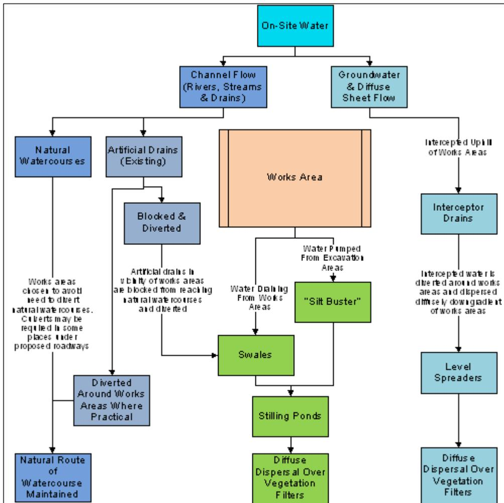
Figure 4-16 Proposed Development Drainage Process Flow
