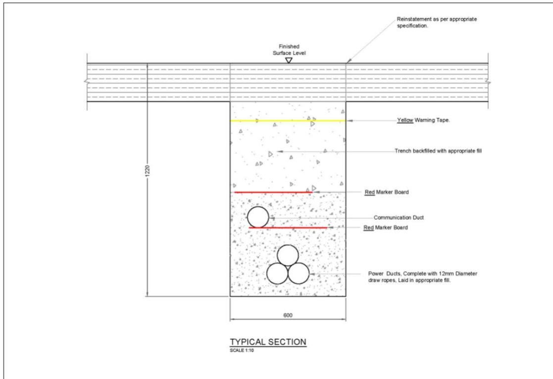
Figure 4-9 Typical Cable trench cross section detail
